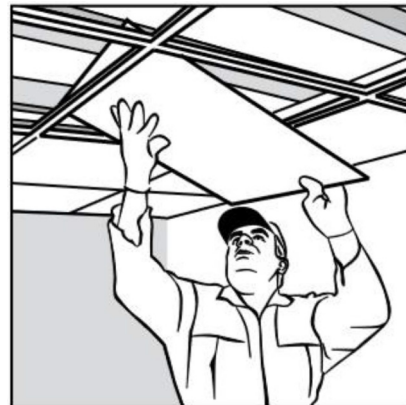
4. Placing the tiles in the grid frames
